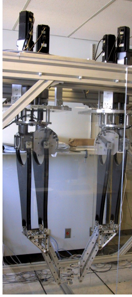
(a) Planetary Gearbox Drive for Double Basal Actuation
