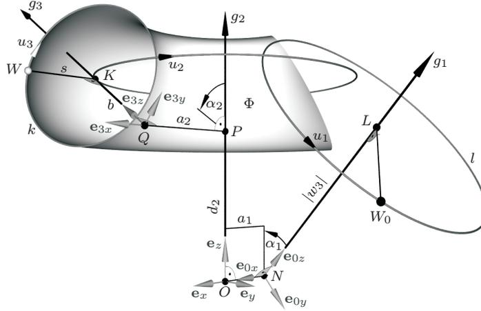
**Fig. 2** The geometric skeleton of the 3R chain with local coordinate systems, the circles  $k$  and  $l$  and a section of the cyclid  $\Phi$ .
