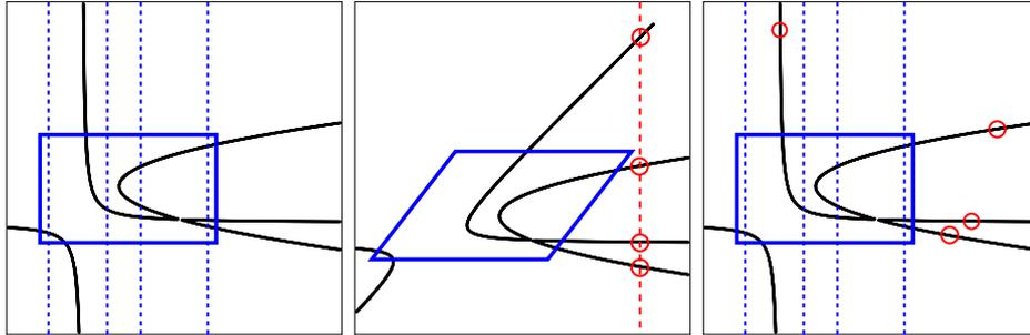
Figure 5.4.2: On the left, the original curve  $f$ . The blue box contains all points where the curve changes the stripe, the stripes are defined by the dashed lines. In the middle, the sheared curve, and the sheared box. The dashed red line on the right corresponds to  $\tau$  in the text. On the right, we see the backsheared points of the sheared points supported by  $\tau$ . We can see the behaviour of the unbounded arc by considering the location of those encircled points.
