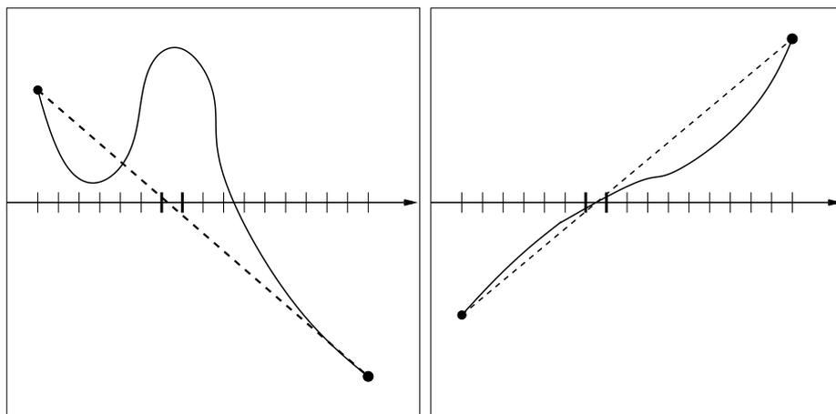
Figure 2.4.1: In the left picture, the guessed interval does not contain the real root, therefore,  $N$  is decreased to 4 in the next step. On the right, there is a sign change in the guessed interval. Therefore, it is taken as refined isolating interval and  $N$  is increased to 256.
