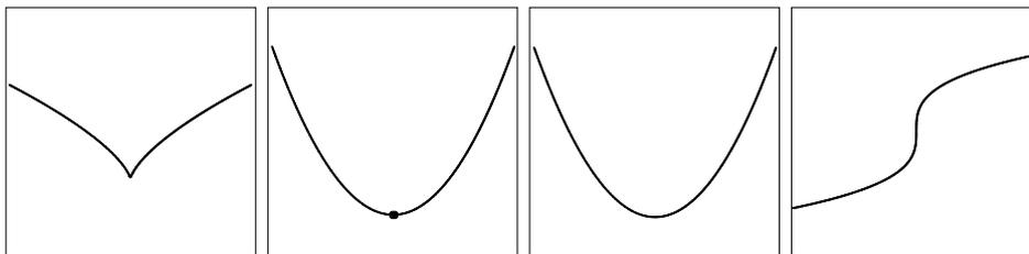
Figure 4.5.1: The curves  $f_1 := x^2 - y^3$ ,  $f_2 := (x^2 - y) \cdot (x^2 + y^2)$ ,  $f_3 := x^2 - y$ , and  $f_4 := x - y^3$ .  $f_1$  and  $f_2$  have singularities at the origin, whereas it is a non-critical point for  $f_3$  and a vertical flex for  $f_4$ .
