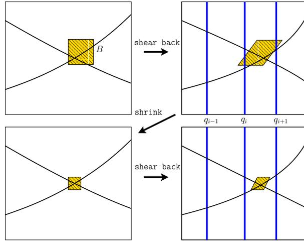
Figure 5.4.1: Above, the box of the event point intersects three stripes. After one refinement, it is completely contained in the stripe between  $q_i$  and  $q_{i+1}$  and hence, the index of this singularity is  $i + 1$ .
