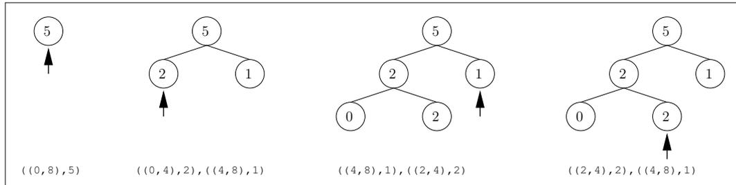
Figure 3.5.1: Example for **Generic Descartes**. It is assumed that the initial interval is  $(0, 8)$  and the split point is always chosen in the middle. The arrow marks the head in the **leaves** sequence, the next processed interval.
