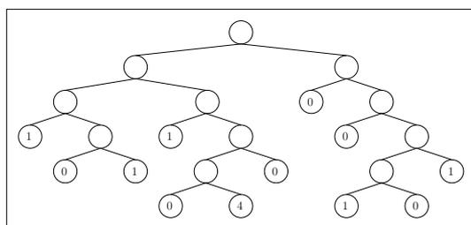
Figure 4.3.1: Assume that we want to find  $m = 5$  roots of the polynomial. In this situation, we found 4 simple roots, and there is only one more interval that with greater sign variation. So the algorithm stops at this point, reporting the five non-zero leaves as isolating intervals.
