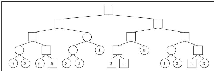
Figure 5.4.3: Let  $e = 4$  and  $m = 10$ . Marked nodes are squares, unmarked circles. The algorithm terminates at this point (and throws away the unmarked interval with variation 2).
