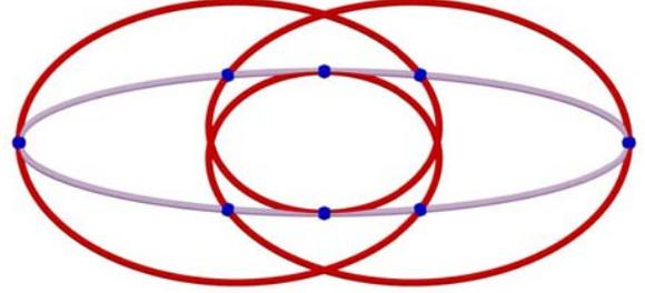
Figure 7: One part of the point paths of  $B_1$  under the self-motions of type A and D.
