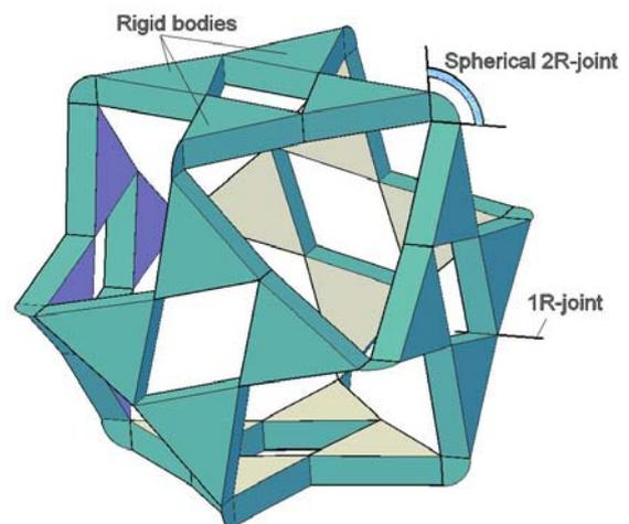
Figure 1: The basic Fulleroid-Like-Mechanism.
