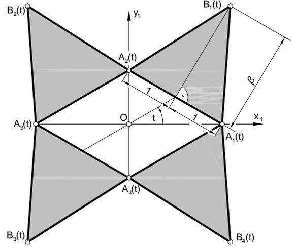
Figure 2: The basic symmetric planar parallel 4-bar.
