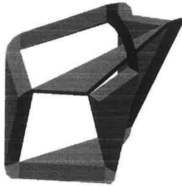
Figure 5. A Möbius mechanism
