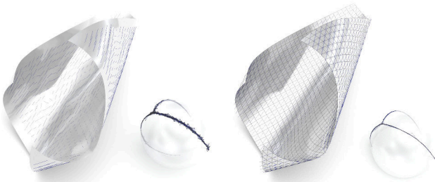
Fig. 24. The mesh on the left has been created using the method of [Rabinovich et al. 2018a]. We illustrate rulings and Gauss image to show that this surface is developable. Further optimization by our method improves the quality (right). The main advantage of our method compared to that of Rabinovich et al. [2018a] is that theirs works with a special parametrization, limiting its capabilities e.g. for modeling.
