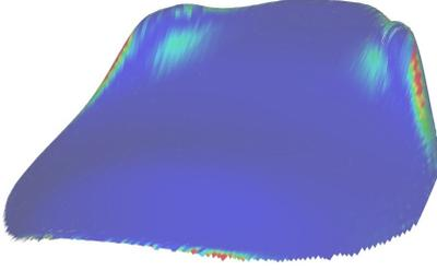
Figure 16: Visualization of Gaussian curvature of the design shown by Figures 11, 12. Blue corresponds to zero, red to the maximum value  $-0.02$  (this means  $\rho = 7.07$ ). The bounding box diagonal of this object is 188.
