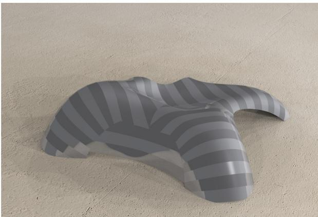
Figure 13: Watertight panels based on the segmentation and parallel transport methods. See also Figure 4. The intrinsic curvature of the rather broad panels is too high to make this design practicable: its purpose is to illustrate the parallel transport method.
