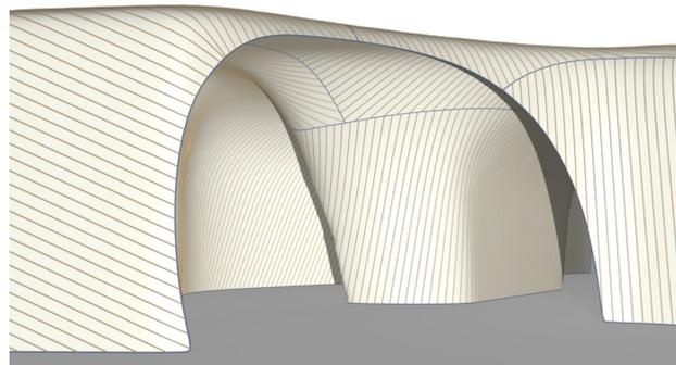
Figure 7: This design with bent rectangular panels is based on Figure 6.
