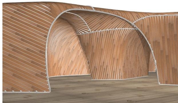
Another idea is that the panel surfaces are *inscribed* into the design surface. For instance we could connect two neighbouring geodesics by a developable surface which is subsequently used for the panel. Algorithmically this is not easy [Rose et al. 2007] and anyway we would rather have a geodesic running in the center of the panel (which is achieved with the idea of circumscribed panels).
