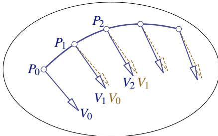
Figure 3: Parallel transport of a vector  $V_0$  attached to the vertex  $P_0$  along the polyline  $P_0P_1P_2\dots$  is algorithmically realized as follows:  $V_i$  is found by orthogonal projection of  $V_{i-1}$  onto the tangent plane of  $P_i$ , and subsequent re-normalizing.
