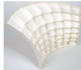
Fig. 18. Kirigami with differently shaped boxes. Optimization has been started from the same base mesh pair, but a different initialization of boxes obviously impacts the shape of the unfolding.
