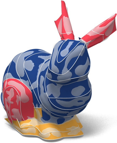
FIGURE 4.13: Approximating the Stanford bunny by composite developable surfaces, using the method of [Tang et al. 2015] not for interactive design, but for fast solution of proximity + developability constraints.
