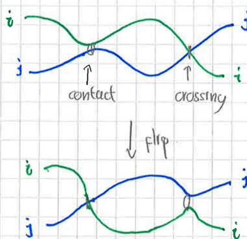
Every contact between two pseudolines  $i$  &  $j$  can be replaced by the corresponding crossing between  $i,j$  (this is unique!) crossing.
