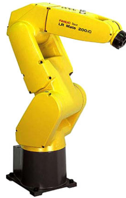
Fig. 2 A very simple 6R robot
