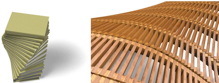
Figure 1: *Conoidal ruled surfaces*. The left hand image symbolically illustrates a conoidal surface, which by definition has rulings parallel to a certain fixed plane. Here spines of stacked books indicate the rulings, which are parallel to a horizontal reference plane. The right hand image illustrates the use of conoidal ruled strips in freeform architectural design: Each strip is made from wooden planks of simple geometry, which are stacked quite in the manner of the stack of books at left.
