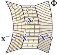
Figure 3: Kinks, resp. absence of kinks in piecewise-ruled surfaces. If strips  $S^-$  and  $S^+$  are to join smoothly in the common point  $\mathbf{x}$ , then the unique tangent plane in  $\mathbf{x}$  must contain both rulings  $\mathbf{x}\mathbf{x}^-$  and  $\mathbf{x}\mathbf{x}^+$ , as well as the tangent vector  $\mathbf{x}_t$  of the boundary curve.
