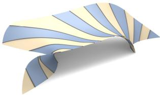
Figure 11: On a detail of the *Cagliari museum project* by Zaha Hadid Architects, strips of constant width have been initialized, but global optimization does not achieve this property. This limitation is due to the fact that strip width is large compared to the size of features of the design surface.
