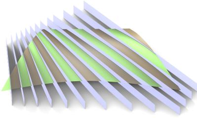
Figure 6: In order to suggest *planar* strip boundaries on a reference surface  $\Psi$ , one intersects  $\Psi$  with a sequence of planes, making sure that the cuts are transverse to a pre-selected family of asymptotic lines (not shown here, but see Figure 5b).
