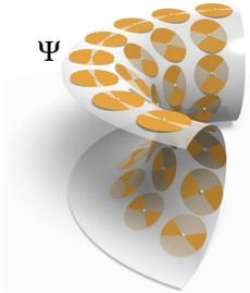
Figure 4: Asymptotic curves in a surface  $\Psi$  have the defining property that their osculating planes (planes spanned by three successive points which converge together) are tangent to  $\Psi$ . It is not difficult to find infinitesimally small segments of such curves, by intersecting  $\Phi$  with its own tangent planes. One can see that only in the negatively curved areas of  $\Psi$  this intersection is meaningful.
