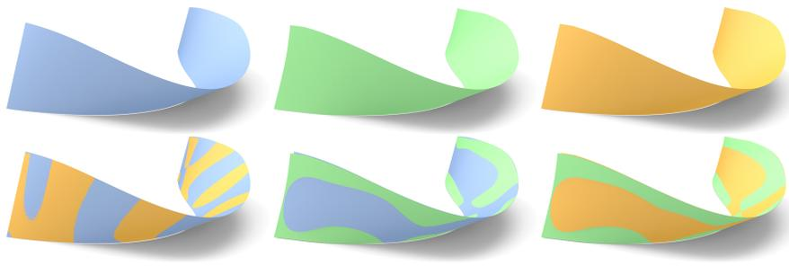
Figure 12: A reference surface (blue) which is an unmodified part of the *Cagliari museum* project by Zaha Hadid architects has been manually initialized and has subsequently been approximated with a single conoidal ruled surface (green) and with a general ruled surface (orange). The bottom row shows these three surfaces superimposed on each other in order to visualize approximation quality.
