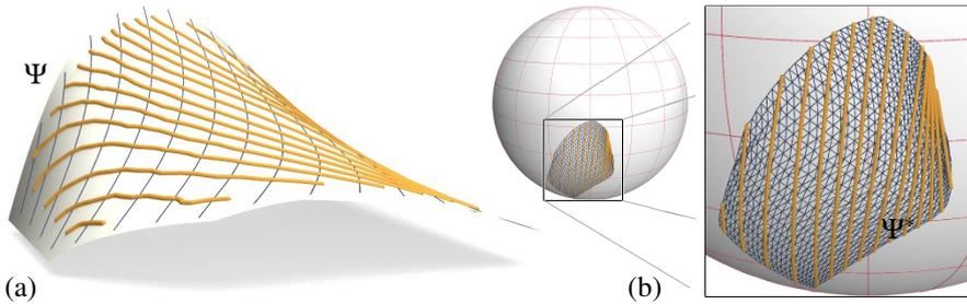
Figure 7: Initializing conoidal strips. (a) Suggested strip boundaries in the mesh  $\Psi$  (yellow). (b) If the mesh  $\Psi$  is mapped to the unit sphere via the asymptotic directions, then strip boundaries are mapped to geodesics in the image mesh  $\Psi^*$  (i.e., to great circles). Note that  $\Psi^*$  is covered by a family of great circles which are in general position to each other, quite unlike the system of meridians of the sphere.
