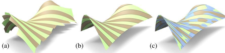
Figure 10: After suggesting strip boundaries as planar cuts through the reference surface (see Figure 6), ruled strips are optimized under the side condition that boundaries are constrained to their respective planes. The result is a watertight union of strips covering the reference surface (a). Subfigure (b) shows the trimmed result. Approximation quality is illustrated by overlaying the reference surface (blue) with the result of optimization in (c).
