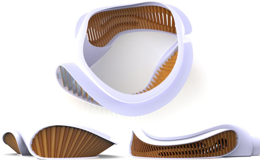
Figure 14: The conoidal ruled strip of Figure 12 serves as the geometric basis of this lamella construction with wooden panels. All panels are parallel to a fixed plane, which is not only a bonus for manufacturing, but has interesting applications with regard to shading. The image at left shows a top view, while the two images below show side views from different directions.
