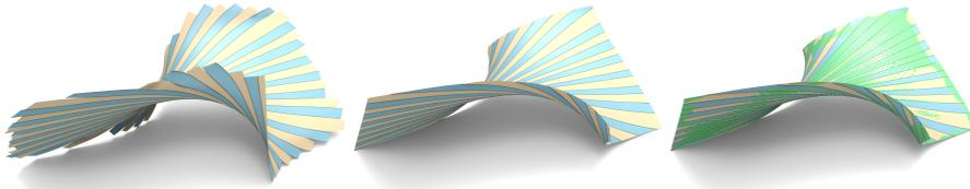
Figure 9: Optimizing ruled strips with geodesic boundaries on part of a so-called “Wohlgemuth-Thayer” minimal surface. From left: optimization result, trimmed result, and illustration of approximation power by overlaying the reference surface. Strip boundaries being geodesic, they can be manufactured by bending wooden panels.
