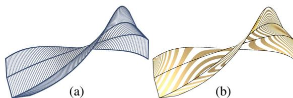
Figure 2: (a) Ruled strips can join smoothly even if their rulings do not. Smoothness is revealed in (b) by continuity of a reflected pattern of zebra stripes.
