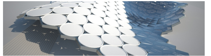
Figure 34: Hexagonal support structure. Here a triangle mesh (not shown) has the property that we can find spheres (shown only by their circular cross-sections) centered in the vertices which touch each other. The common tangent planes of these spheres are the faces of a support structure (visible at boundary in front). This is part of a design created by H. Schmedhofer for [88].
